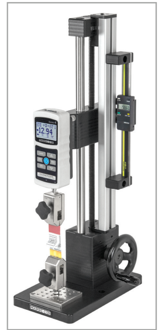
▲ Shown with an ES30 test stand and G1008 film & paper grips
