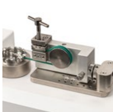
Fig. 3.5 Bollard grip assembly (optional)
