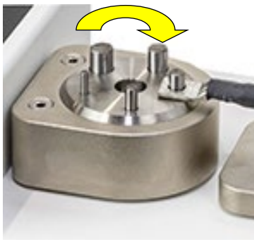
Fig. 3.2 Ring terminal fixture (optional)
