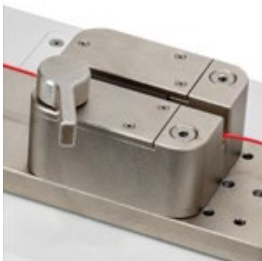
Fig. 3.4 Wedge grip assembly (standard, mounted to actuator)
